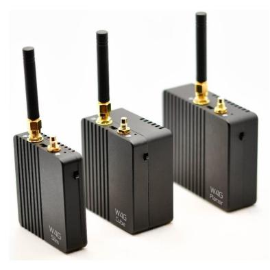
Wave4G is a Video, Audio, Gps store&forward unit, stereo, miniaturized and has been developed for covert surveillance use.
