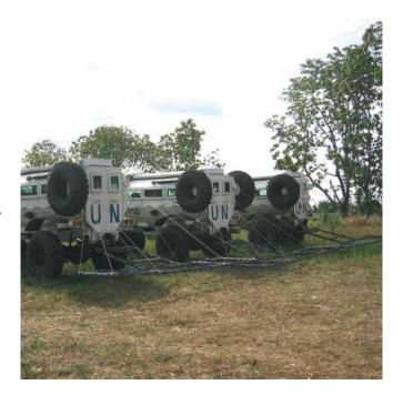
UPEX® 740 MVM triple system used in road inspection
