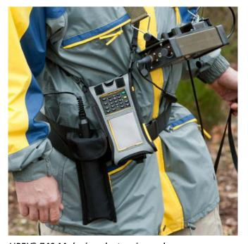
UPEX® 740 M device electronics and EPAD® data logger
