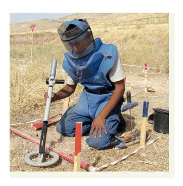
EBEX® 422 GC, most advanced detector for minimum amount of metal mines
